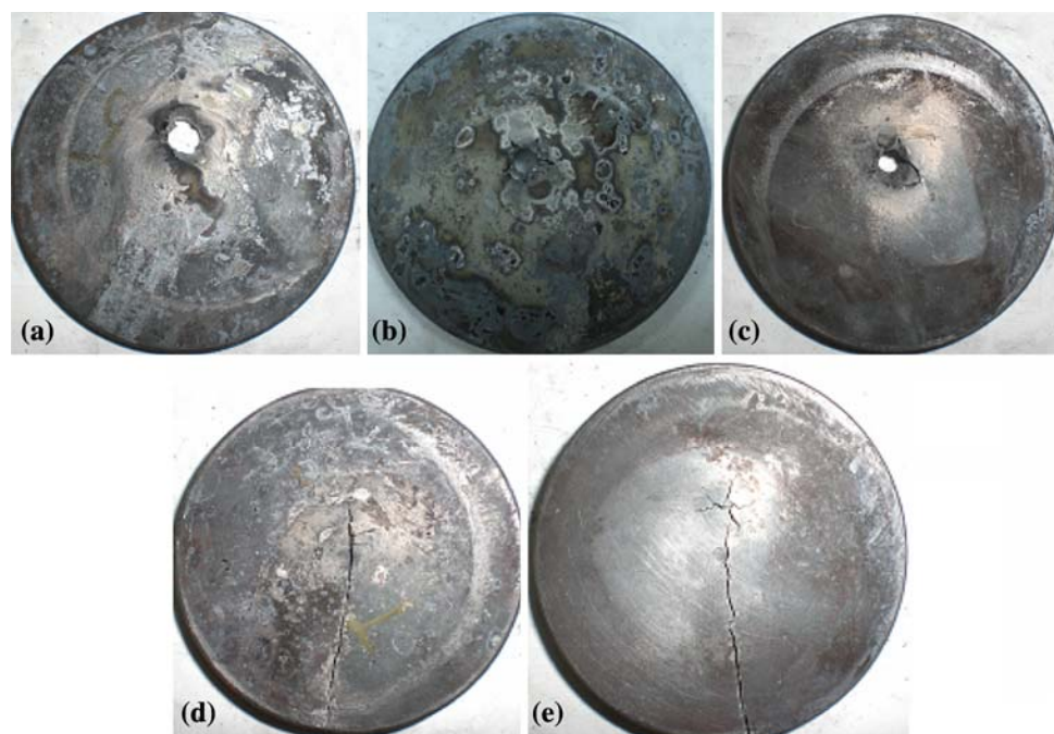
Fig. 7 Rear view of the specimen group 2A: (a) 2A1, (b) 2A2, (c) 2A3, (d) 2A4, and (e) 2A5. It is apparent that the specimens 2A4 and 2A5 were not perforated by the projectiles but only a radial crack was formed at the rear side of the specimens
